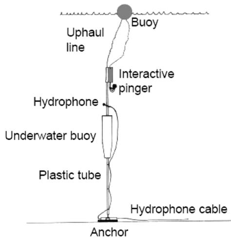
*Figure 2. The sketch demonstrates the pinger deployment setup, which keeps each pinger steady in the array and at the same level above the bottom (2.2 m).*
